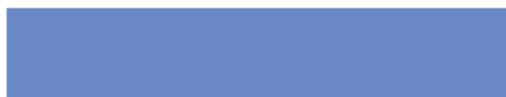
Fig. 2 A dielectric slab with flat surfaces. The thickness is equal to the equivalent thickness of the structure in Fig. 1 so the two structures contain the same amount of absorbing materials.
