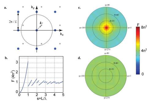
Fig. 5. a) Channels in 2D k-space. Blue and grey dots represent channels when the incident light comes in from normal and off-normal directions, respectively. The radius of the circle is  $k_0$ . b) Limit of absorption enhancement in 2D grating structures. c) Angular response of the average enhancement factor integrated over wavelength from 600nm to 1200nm. The periodicity of the grating is 600nm. d) the same as (c) except the periodicity is 3000nm.
