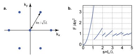
Fig. 7. a) Channels in 2D k-space for a grating with triangular lattice periodicity. The lattice constant is L b) Upper limit of absorption enhancement for gratings with triangular lattice periodicity.
