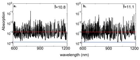
Fig. 4. Absorption spectra for off-normally incident light (averaged among s and p lights). Light incidence angle is  $30^{\circ}$  and incident plane is oriented at azimuthal angle  $30^{\circ}$ . a) for the asymmetrical structure in Fig. 1a. b) for the symmetrical structure in Fig. 3a.
